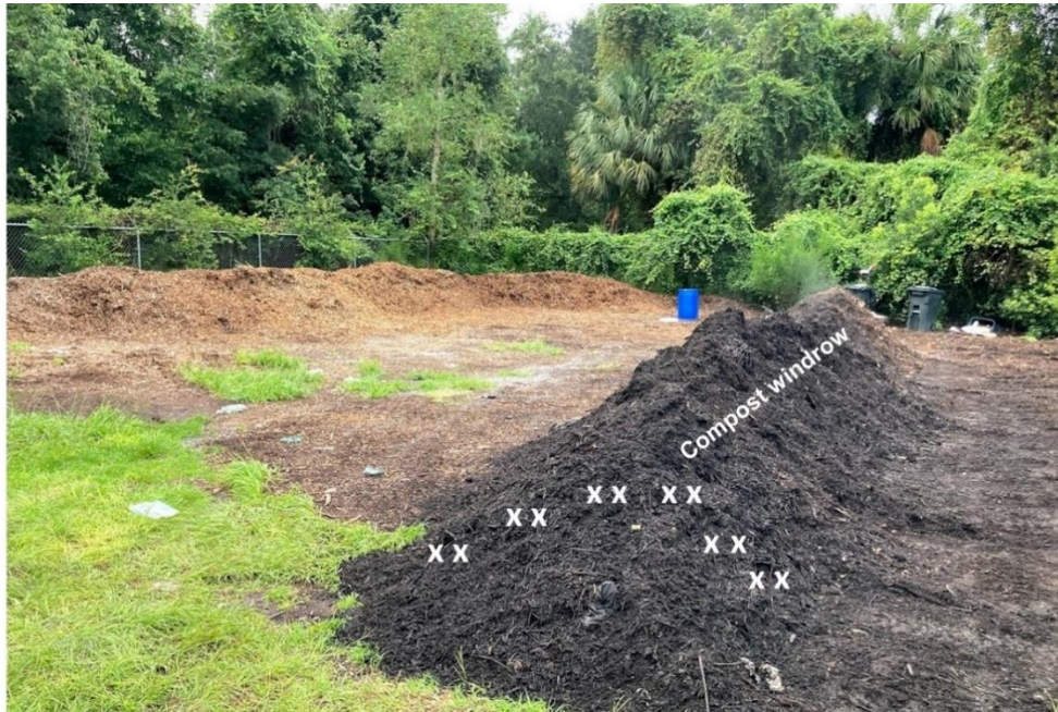
Figure S1. Composite compost sampling scheme. Each mulch and compost sample was a composite of 12 scoops: two scoops each from the top, middle and bottom of the pile, on both sides of row. An example compost windrow sample is illustrated here. Each “X” represents one scoop. The top layer of material was moved aside before samples were scooped at an approximate depth of six inches below the surface of the pile.
